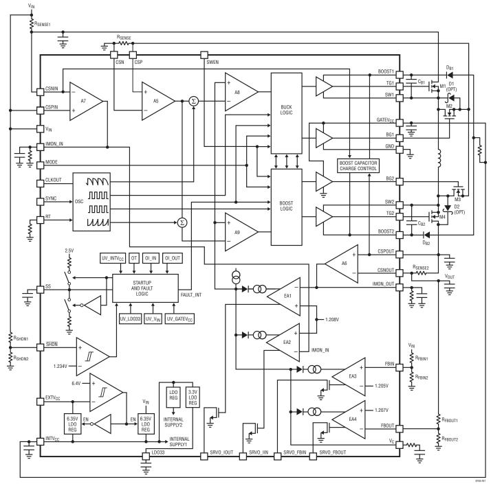
Figure 1. Block Diagram
