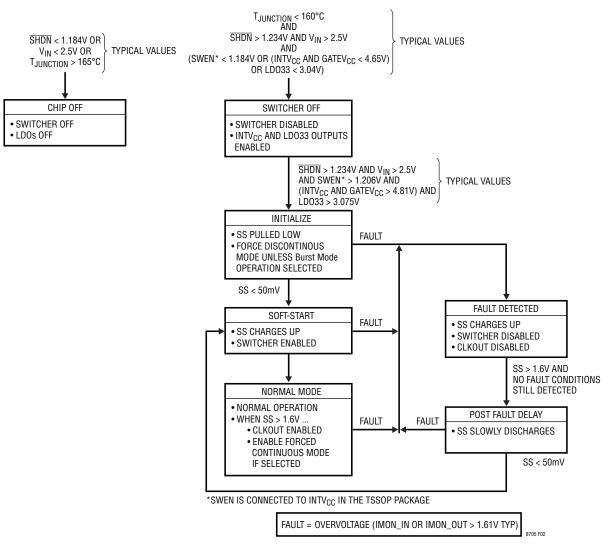
Figure 2. Start-Up and Fault Sequence
