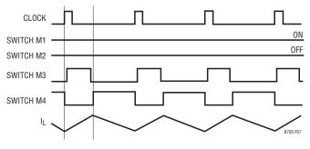
Figure 7. Boost Region ( $V_{IN} \ll V_{OUT}$ )
