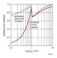
Figure 8. Currents vs V<sub>IN</sub>/V<sub>OUT</sub> Ratio
