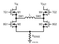
Figure 3. Simplified Diagram of the Output Switches
