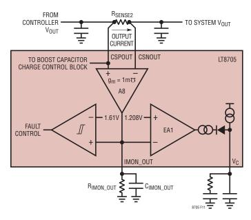
Figure 11. Output Current Monitor and Limit
