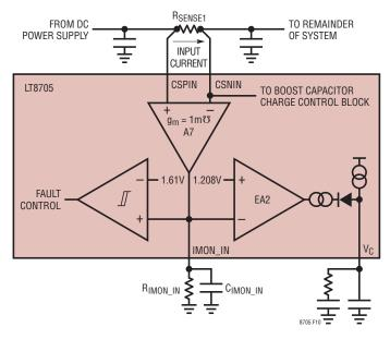
Figure 10. Input Current Monitor and Limit
