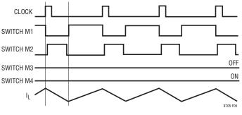
Figure 5. Buck Region ( $V_{IN} >> V_{OUT}$ )
