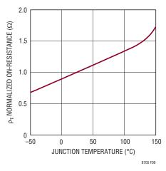
Figure 9. Normalized MOSFET R<sub>DS(ON)</sub> vs Temperature
