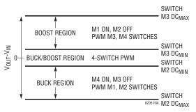
Figure 4. Operating Regions vs  $V_{OUT}$ - $V_{IN}$
