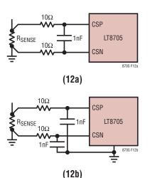
Figure 12. Inductor Current Sense Filter
