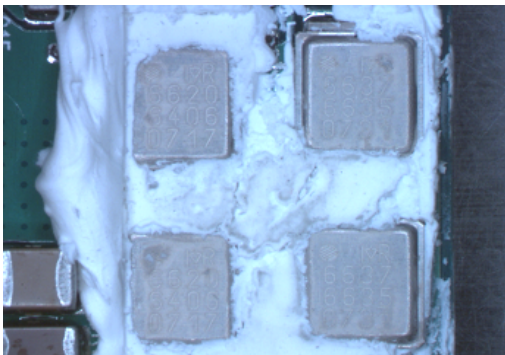
Figure 15 Excess heatsink adhesive covering devices
