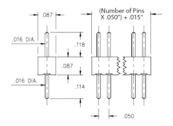
**Description:** Interconnect Header .050 Grid; Straight Pin Header Single Row Through Hole Plating Code:
