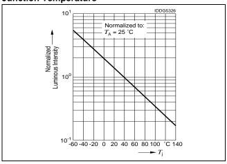
When mounted in a 10°C/W socket and operated at Absolute Maximum Electrical conditions, the HDSP200XLP will show an LED junction rise of 17°C. If  $T_{\rm A}$ =40°C, then the LED's  $T_{\rm J}$  will be 57°C. Under these conditions the following figure shows that the  $I_{\rm V}$  will be 75% of its 25°C value.
